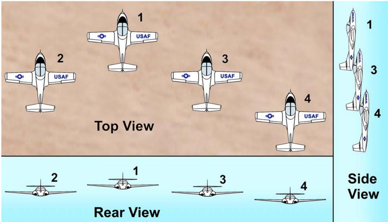
Figure 8.25. Four-Ship Fingertip Formation in a Turn.
